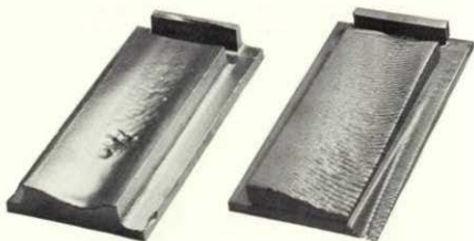
At left — Long-Lyfe Liner after 731 hours. The other is a Sibley Liner after only 38 hours service.
